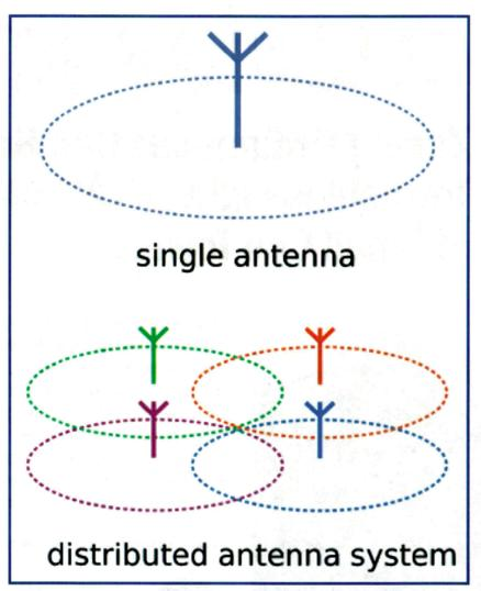
Rather than relying on a single, traditional cell tower located in a remote area, wireless carriers are installing distributed antenna systems. These consist of numerous smaller structures that cover a targeted area, such as a neighborhood. (Diagram by Tod Robbins/Wikimedia Commons/Public Domain.)
